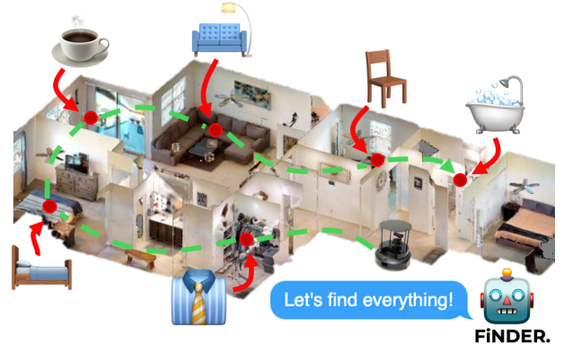
Fig. 1. Finder utilizes a vision language model to address the multi-object search problem for a mobile robot in any indoor environment.
